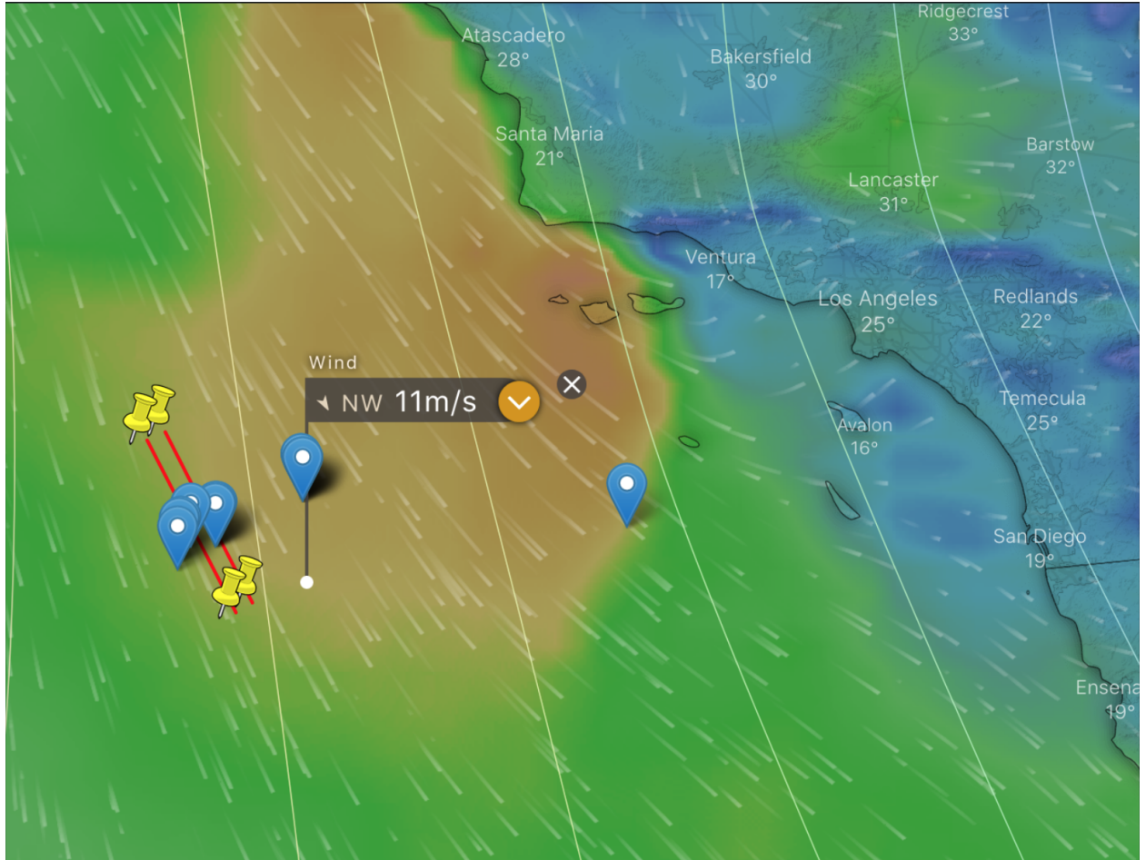
Figure 2: Wind conditions during the May 18 deployment. The B200 TFO lines are shown in red and the markers show the location of the in situ assets. The winds ranged from below 3 m/s to above 12 m/s during the flight.
