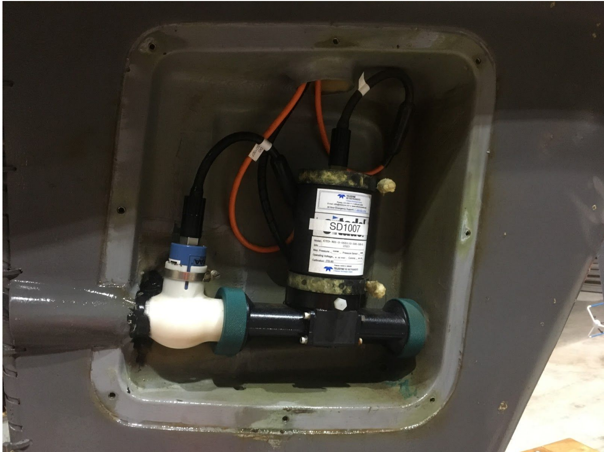
Figure 12. Dissolved Oxygen sensor installed on a Sailandrone.
