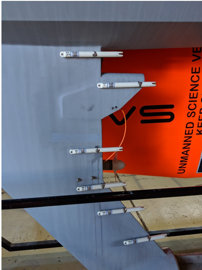
Figure 3. Installation of temperature loggers along keel.
