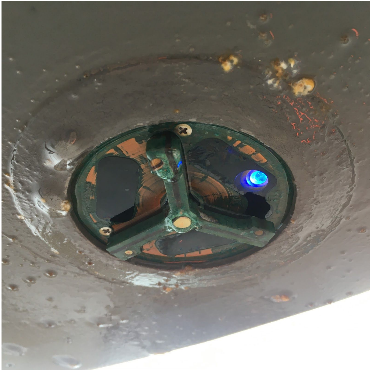
Figure 20. ADCP installed on a Saildrone vehicle.
