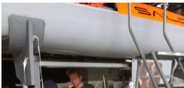
Figure 21. ADCP installed on a Saildrone (vehicle rotated 90 degrees to present the bottom of the hull).
