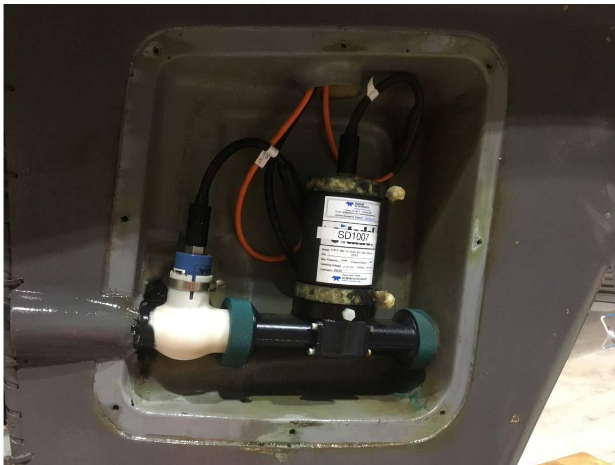
Figure 12. Dissolved Oxygen sensor installed on a Saildrone.
