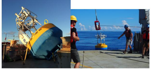
Figure 3.48. Central mooring onboard Revelle during cruise 2 (left). Central mooring being deployed from Revelle into the Pacific Ocean during cruise 2 (right).
