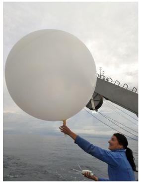
Figure 3.32. A rawinsonde being released off the aft deck of the Revelle during cruise 2. Image courtesy of Ben Greenwood.
