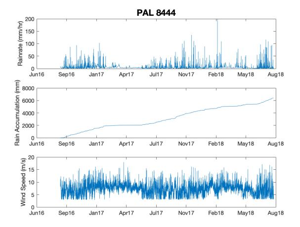
Figure 3.102. Rainrate, rain accumulation, and wind speed of the PAL 8444 sensor.
