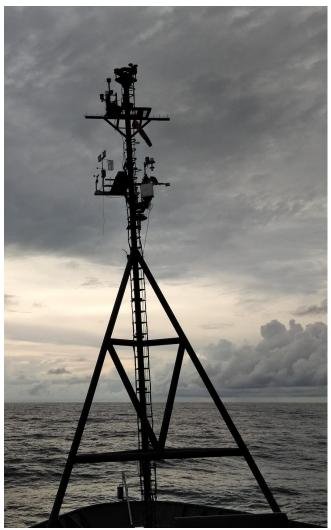
Figure 3.28. Meteorological instruments on a mast mounted on the bow of the Revelle on cruise 2. Photo courtesy of Ben Greenwood.
