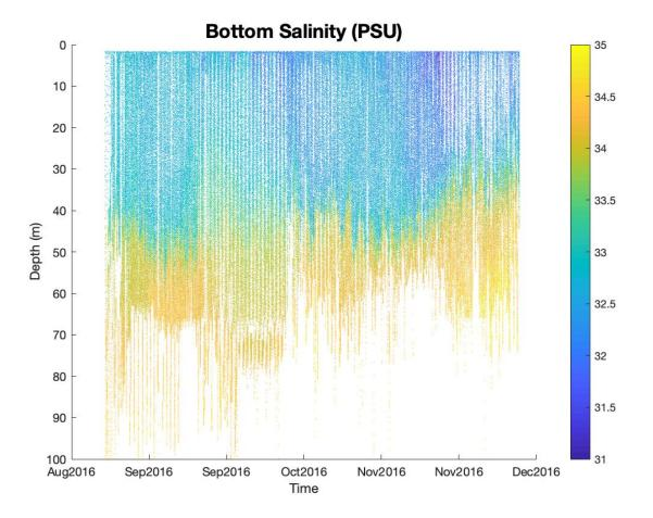
Figure 3.88. Seawater salinity from the bottom sensor of the Sea-Bird Scientific SBE 41 CTD.
