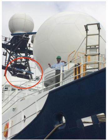
Figure 3.45. The mast of the Revelle, and the SEA-POL radar. The X-band radar is circled. Image courtesy of E. Thompson.
