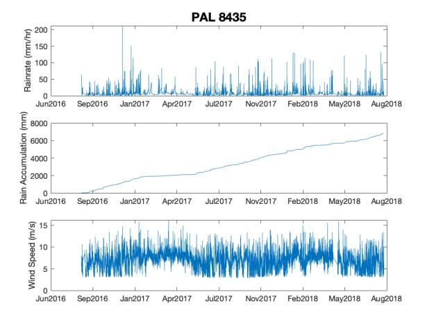
Figure 3.101. Rainrate, rain accumulation, and wind speed of the PAL 8435 sensor.
