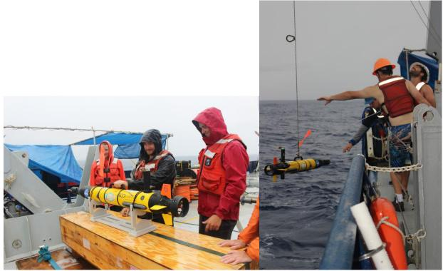
Figure 3.42. EcoMapper being deployed from the Revelle. Photo courtesy of Spencer Kawamoto.
