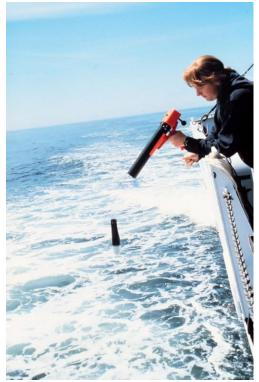
Figure 3.18. Expendable bathythermograph (XBT) being launched from a vessel (<u>Wikimedia</u> <u>Commons 2019</u>).
