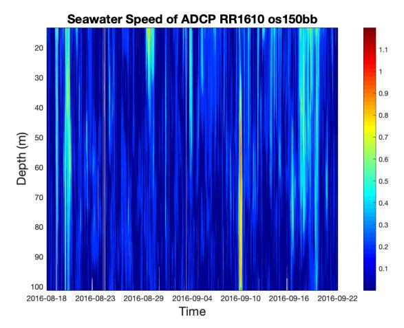
Figure 3.5. Seawater speed (m/s) with depth of ADCP os150bb during Revelle cruise 1.
