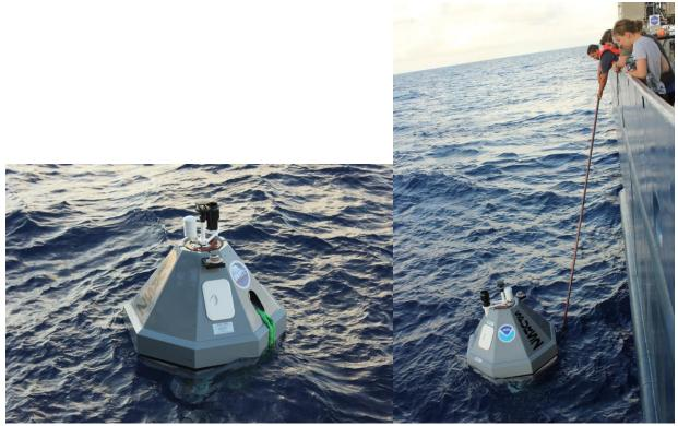
Figure 3.51. Retrieval of PICO mooring from the Revelle. Photo courtesy of A. Jessup.
