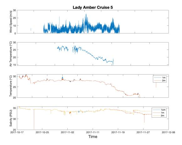
Figure 3.108. Wind speed, air temperature, seawater temperature at 1m and 2m, and seawater salinity at 1cm, 1m, and 2m collected during Lady Amber's cruise 5.
