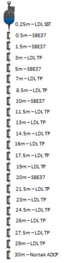
Figure 3.65. The configuration of the SADOS drifter. Each LDL TP measured temperature and pressure. Each SBE73 measured temperature, conductivity and pressure. The ADCP at 30 m was upward-looking. Figure courtesy of V. Hormann.
