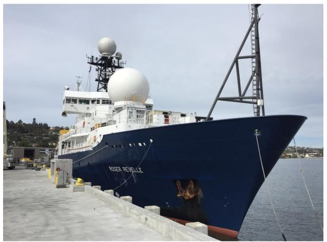
Figure 3.43. The Revelle in port in San Diego prior to cruise 2. The SEA-POL radar is the large "golf ball" radome placed in front of the bridge on the 02 deck.
