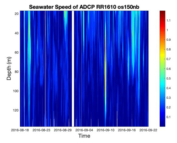
Figure 3.7. Seawater speed (m/s) with depth of ADCP os150nb during Revelle cruise 1.
