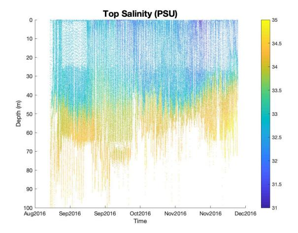
Figure 3.87. Seawater salinity from the top sensor of the Sea-Bird Scientific SBE 41 CTD.
