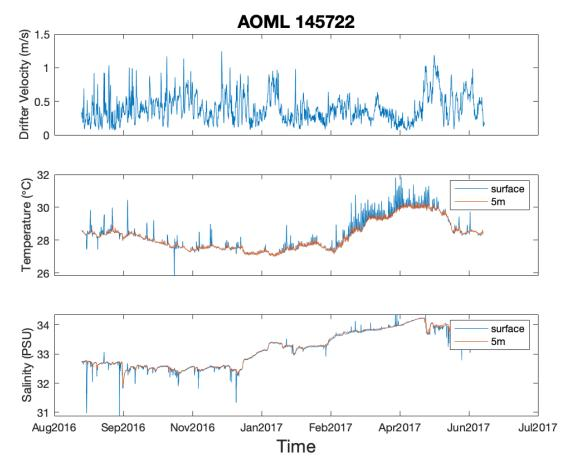
Figure 3.82. Drifter velocity, seawater temperature at the surface and at 5m, and seawater salinity at the surface and at 5m from AOML drifter 145722.
