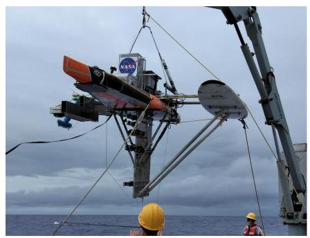
Figure 3.27. The SSP being deployed off the side of the Revelle on 30-Oct-2017. Note the keel with three CTDs on the left side and two microstructure probes on the right. The intake for the
