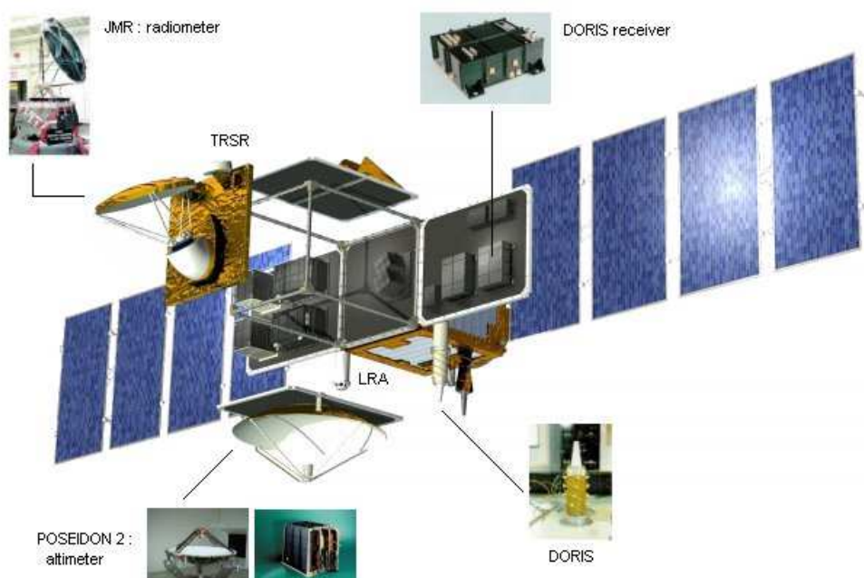
Figure 2 : Main components of the Jason-1 satellite
