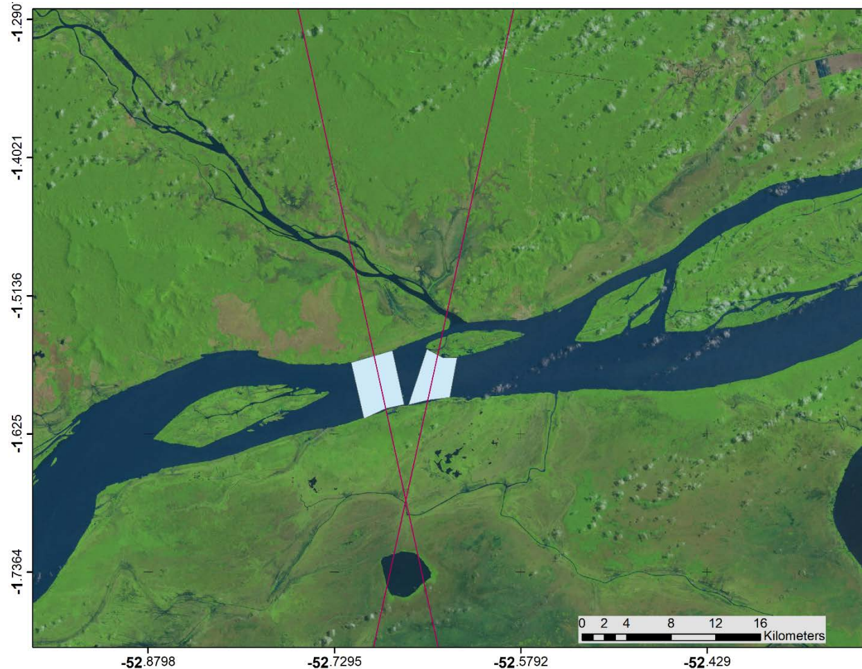
Figure 2 A sample Landsat Scene from the Amazon River with to VS polygons and their overlying Envisat ground tracks.
