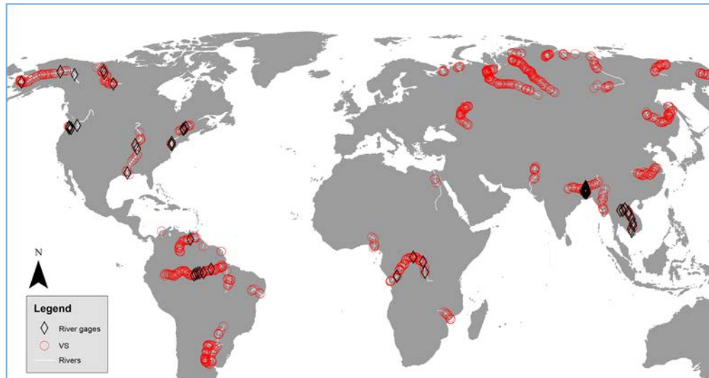
Figure 3 VS and validation sitemap. Red circles show locations of 9020 virtual stations. Black triangles show the locations of 50 validation gauge locations.
