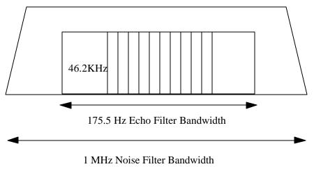
Figure 5-1 Illustration of Slice Resolution for 0.5msec Effective Gate Width
