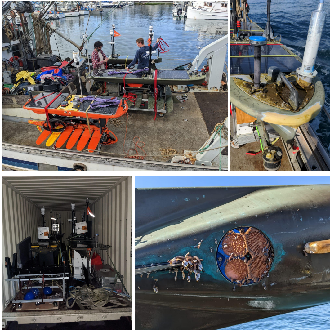
Wave Glider recovery on November 7 2022 from the F/V Shana Rae. Note the biofouling after the 7+ weeks long deployment.
