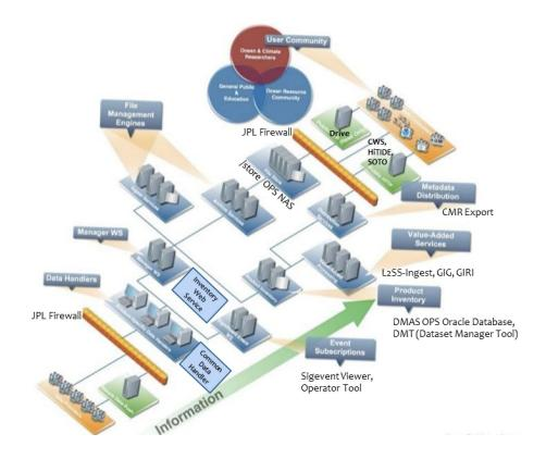
Figure 1. Architecture schematic of the PO.DAAC capturing the external interfaces for data ingestion and monitoring, internal data and metadata storage, and public consumption of data and services.
